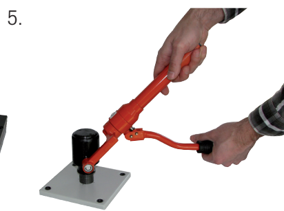
Pilot hole - For bolt \varnothing 9.5 mm, with \varnothing 10.5 mm - For bolt \varnothing 11.1 mm, with \varnothing 12 mm - For bolt \varnothing 19 mm, with \varnothing 20 mm, for bolt \varnothing 19 mm you can also pre-drill a \varnothing 20.4 mm hole - For shaped punches: use largest bolt diameter +1.5 to 2 mm
