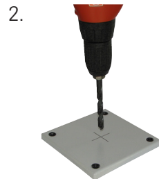
Pilot hole - For bolt \varnothing 9.5 mm, with \varnothing 10.5 mm - For bolt \varnothing 11.1 mm, with \varnothing 12 mm - For bolt \varnothing 19 mm, with \varnothing 20 mm, for bolt \varnothing 19 mm you can also pre-drill a \varnothing 20.4 mm hole - For shaped punches: use largest bolt diameter +1.5 to 2 mm
